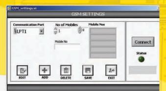
Keeps track of temperature and humidity Alerts user via SMS on high/low temperature and humidity Connects up to five mobiles
